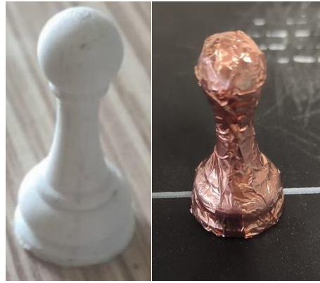
Figure 3. Printed design and covered with copper tape
